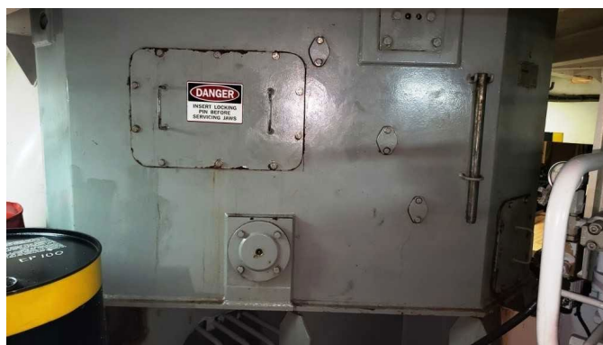
Figure 3. – Shark jaws inspection cover on Bourbon Rhesos 4
