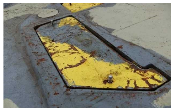
Figure 2. - Retracted shark jaws on Bourbon Rhesos 3
