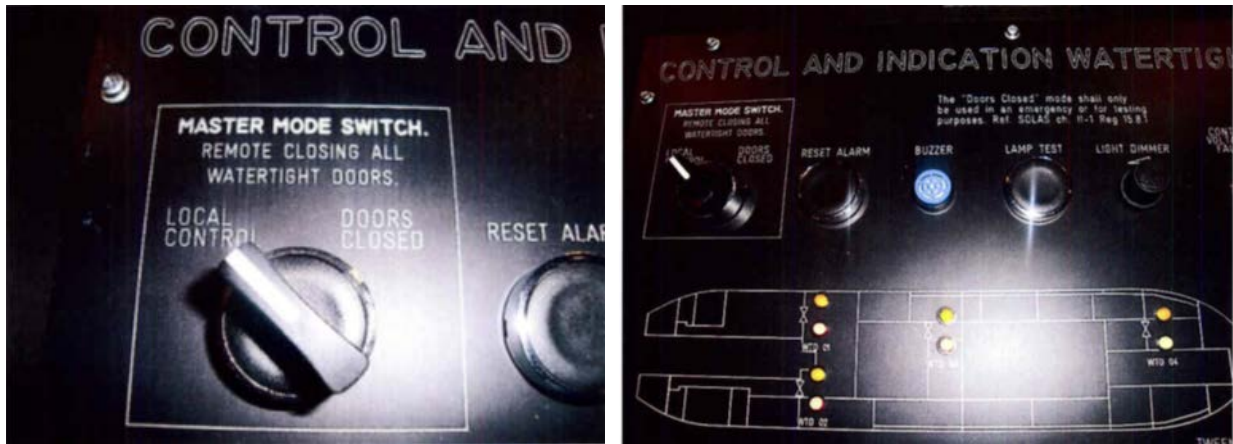
Figure 3.6 – Control and indication panel of the WTDs' system (Source: Schoenrock Hydraulik Marine Systeme GmbH)
