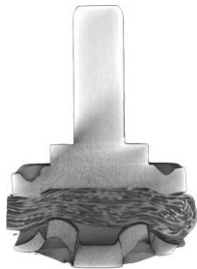
Figure 15. Terminal (J) power braid wire crimped
