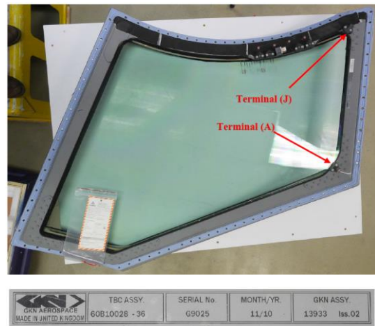
Figure 3. R1 Windshield s/n G9025 inside view and data tag
