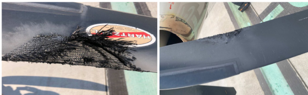
Figure 2: Damage observed on a propeller blade
