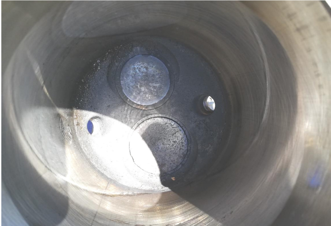
Figure 2: Combustion residues on the intake and exhaust valves of cylinder no. 3.
