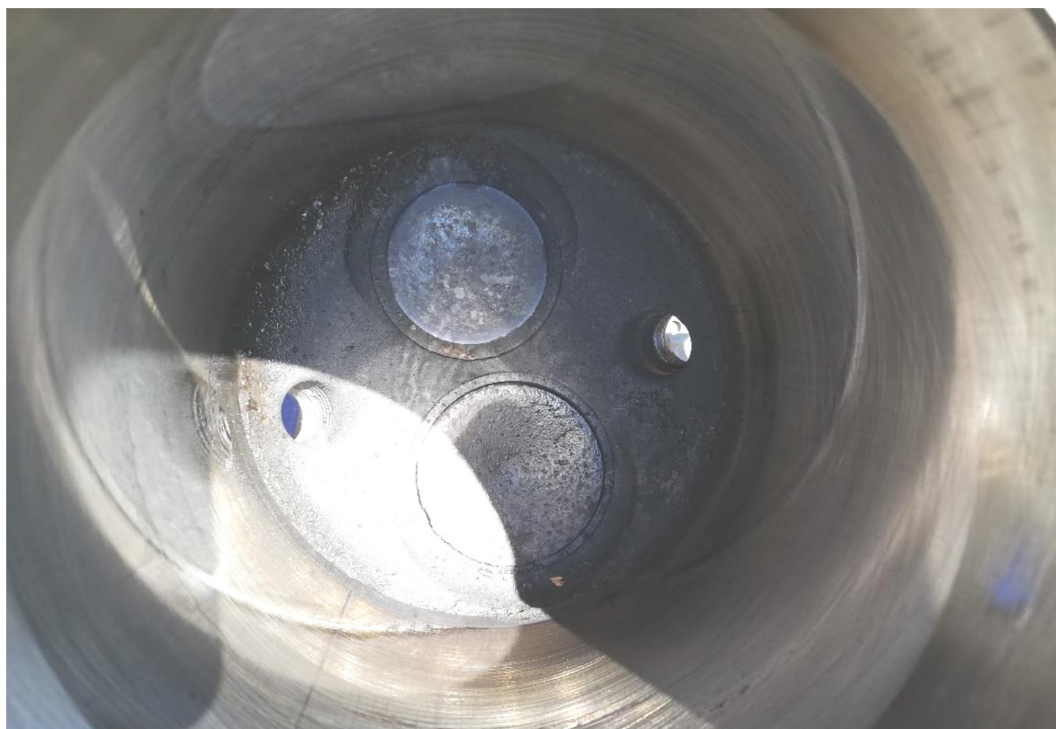
Figure 2: Combustion residues on the intake and exhaust valves of cylinder no. 3.
