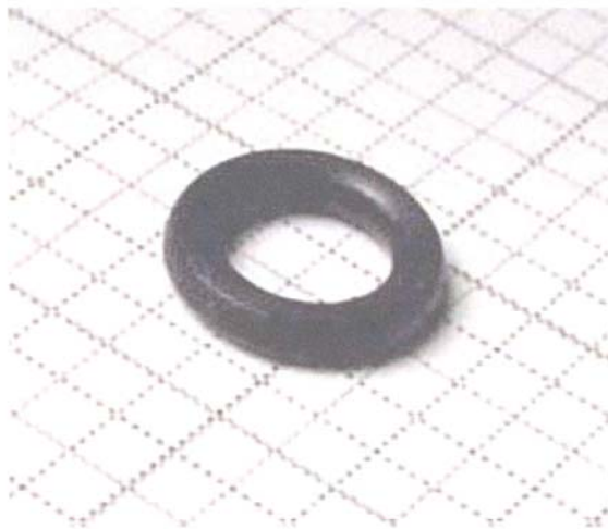
Figure 10 – C2 Filter Seal
