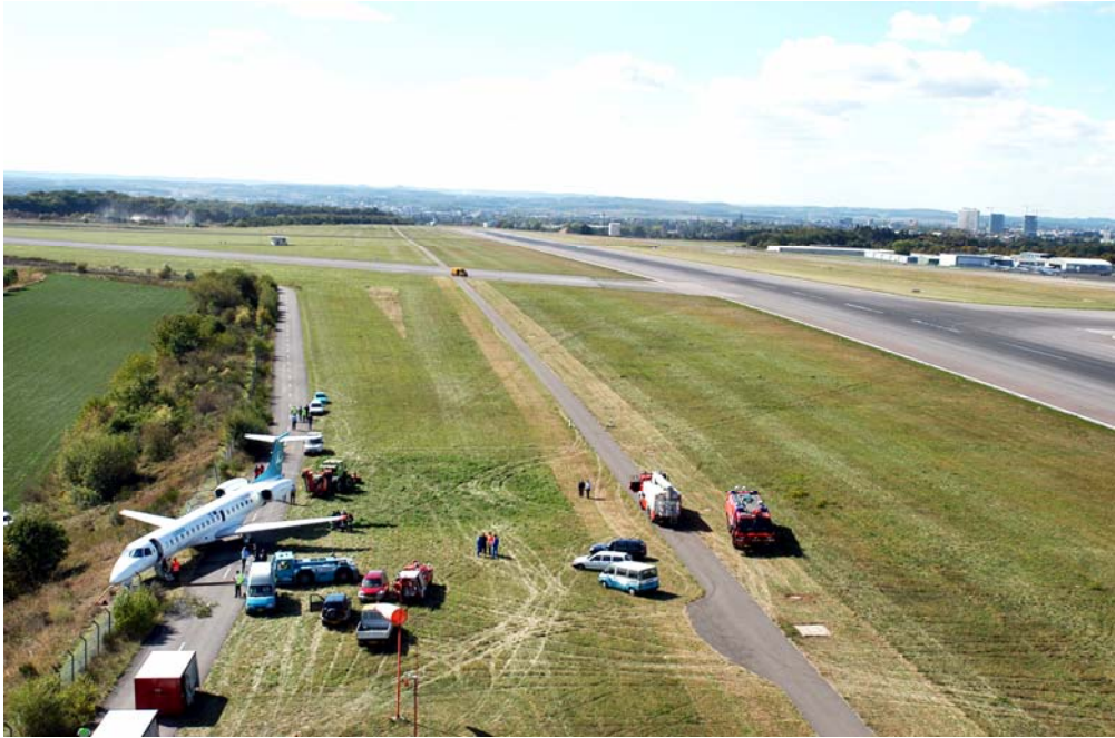
Figure 2. Aircraft was arrested by the airport boundary fence
