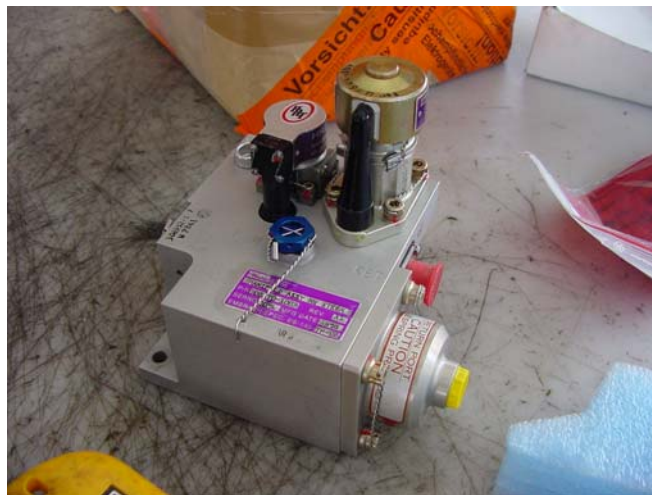
Figure 16. NW steering hydraulic manifold SN 0096
