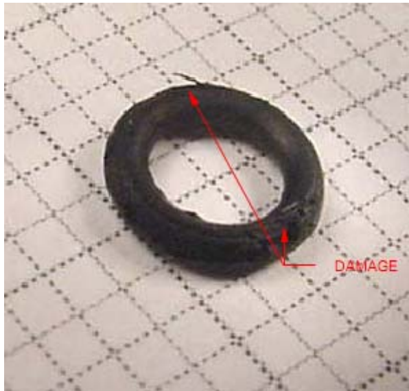
Figure 20. C1 Filter Seal
